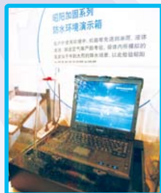
具有防水防尘、抗振抗压、抗跌落抗冲击特性的加固笔记本电脑 The reinforced computer With the characteristics of waterproof and dustproof, vibration resistance and compression resistance, anti-drop impact
